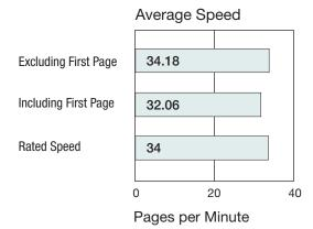
Print speed is tested using BLI's Monochrome Test Original with 6% page coverage. The test page is printed in a quantity equal to double the vendor's rated print speed for the device in each mode tested (e.g., if the vendor's rated print speed is 20 ppm, 40 pages are printed). The unit's print speeds were tested using the PCL driver.
