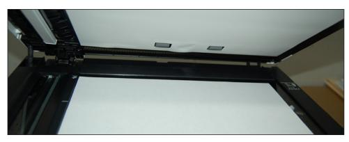
The page is scanned in two halves (grey rollers, shown above, in the platen cover automatically move the page so no user intervention is required) and then digitally combined in the device memory; output is automatically resized to a letter-size page. Though 11" x 17" isn't frequently used, this innovative device gives users the ability to scan and copy these larger pages on a compact and affordable device.
