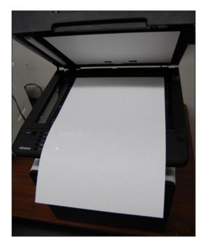
A unique feature of the M402dn lets users copy an  $11^{-x-17}$  page by placing it on the platen and pressing the A3/11 x 17 START button (rather than the start key, which is covered by the page) to initiate the copy.
